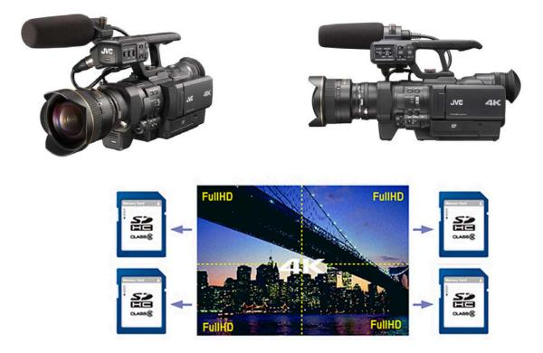
To demonstrate 4K encoding we decided to use the JVC GY-HMQ30 along with our HCoder Quad<sup>™</sup> (with 4 channel H.264 encoder with mux), and a D-Streamer Magnus IP<sup>™</sup> / Dig Quad. As a first step we elected to test the decoding output on a 4 HD input quad LCD monitor. A 4K monitor or Display plus a media processor or blender like the Sony MPE 200, AnalogWay Ascender, or Vista Systems Spyder would have presented a non segmented picture but none were available at the time of testing.
