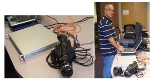
We took the 4 HDMI 1080p60 (1 per quadrant) from the JVC camera and fed the Quad Encoders 4 inputs. The Quad encoded each input/ quadrant to 6.5 mbps H.264 UDP. The 4 6.5 mbps streams were then multiplexed (muxed) into a single 30 mbps (null packets included to help with delivery).
