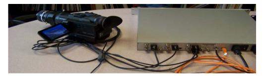
Out of the Quad Encoder the muxed IP (quad 1080 videos) went to the decoder Quad Via IP and Internet. The decoder Quad demultiplexed the streams into individual HD-SDI channels that were all in sync. These 4 Channels were displayed on a quad 1080p display. So each quadrant was labeled. We wanted to see any movement from quadrant to quadrant.
